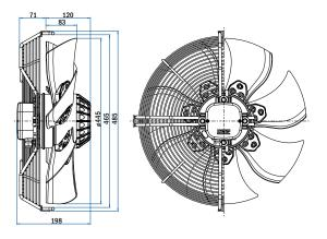
Fan characteristic measured in full bell mouth with guard grill. ErP characteristic measured in full bell mouth without guard grill.
